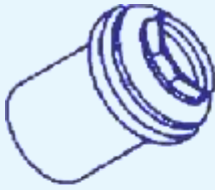
COUPLING FLANGED No. M110/M111 S. No. : O 154 Size : 20mm 25mm 32mm Material : Malleable Iron Pack Qty : 50 50 25
