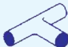
TEE S. No. : O 159 Size : 20mm 25mm 32mm Material : Malleable Iron Pack Qty: 25 25 10
